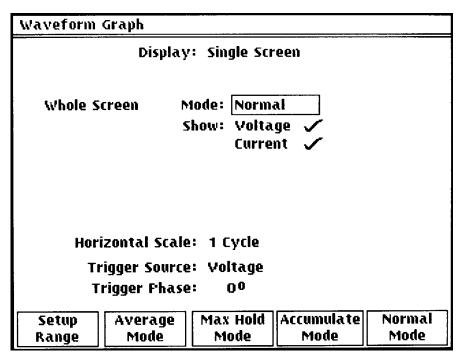
With the exception of the Setup Range key, the functions of the soft-keys change as the edit zone is moved through the editable fields of the display using the ▲ ▼ keys; each field is described below. Pressing the VIEW key returns the display to the Waveform Graph view.
