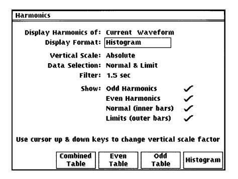
The soft-key functions change as the edit zone is moved through the editable fields of the display using the ▲ ▼ keys; each field is described below. Pressing the VIEW key returns the display to the Harmonics view. The selections made for each of the display formats are stored until the instrument is switched off.
