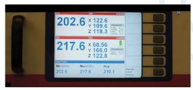
The SY3-EMC has been tested at all required frequencies between 30 and 200 MHz in both horizontal and vertical positions. Typical results in a fully anechoic test chamber in horizontal configuration\*:
