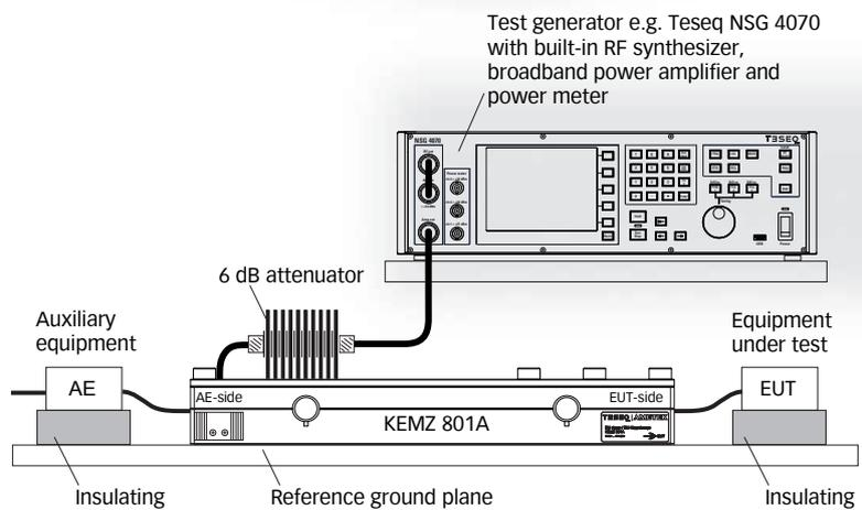
Test set-up with EUT according IEC / EN 61000-4-6 with EM clamp and monitoring probe
