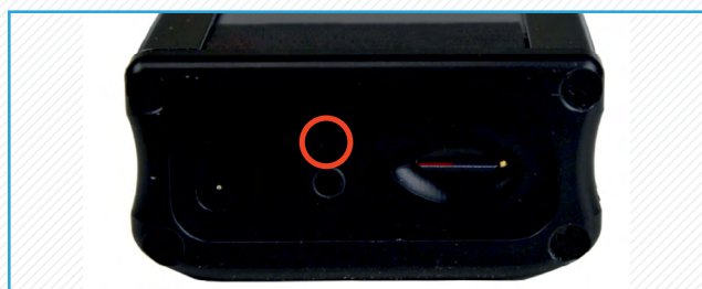
Figure 7. Location of the reset button at the bottom of the ESD Event Meter
