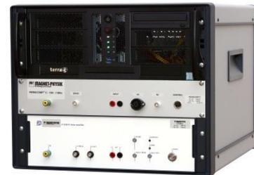
Cabinet of REMACOMP<sup>®</sup> C - 100 - 1 MHz, housing power amplifier and computer
