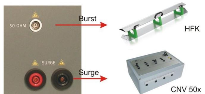
Figure 3.1: External device plug for Burst and Surge
