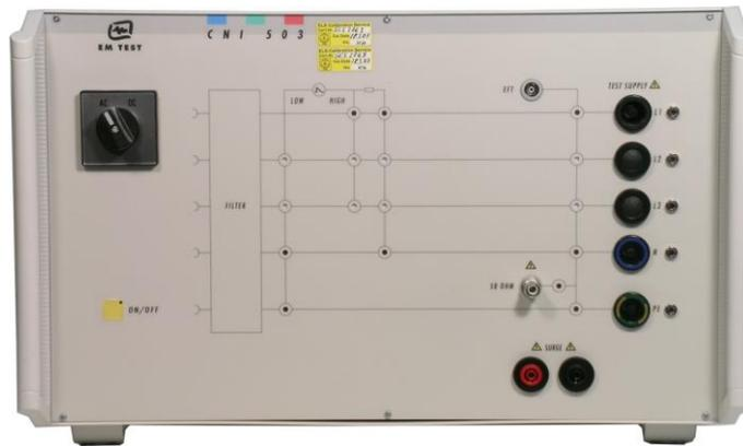
Figure 2.3: Front side CNI 501 S1 with AC / DC switch
