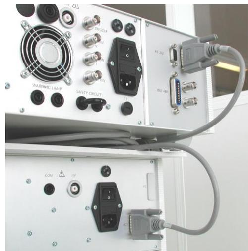
Figure 6.4 : Connection the CN cable
