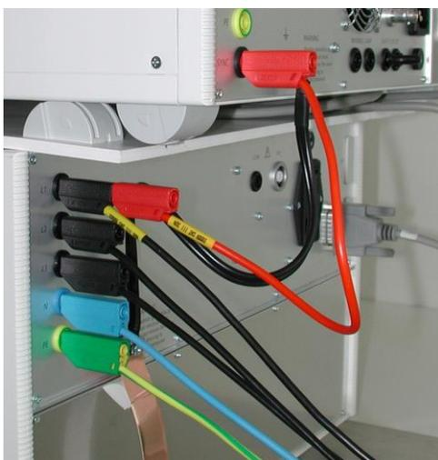
Figure 6.3 : Connection line power and sync to UCS 500
