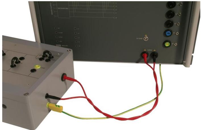
Figure 6.8: Connection of a CNV 504 to a CNI 503
