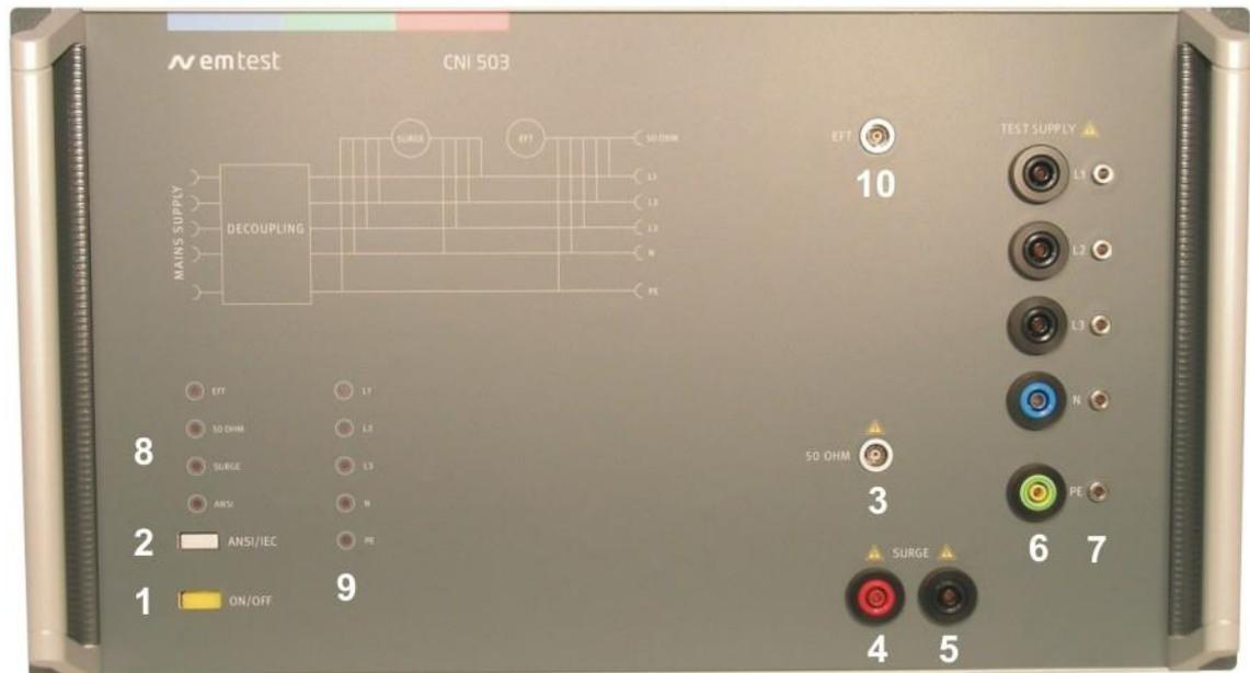
Figure 2.1: CNI 503 front view ( model for 4kV )
