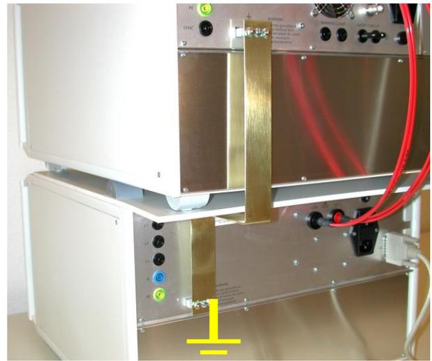
Figure 6.7: Earth connection with brass plate
