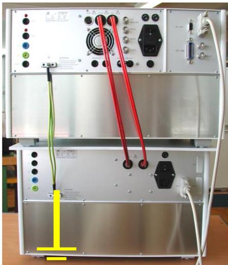
Figure 6.6: Earth connection with cables
