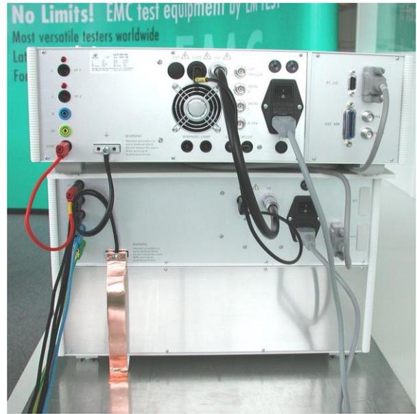
Figure 6.5 : Connection to reference ground
