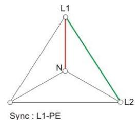
Figure 5.1 Phase shift between star and delta
