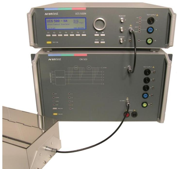
Figure 6.9: Connection of a capacitive coupling clamp to the UCS 500 M4
