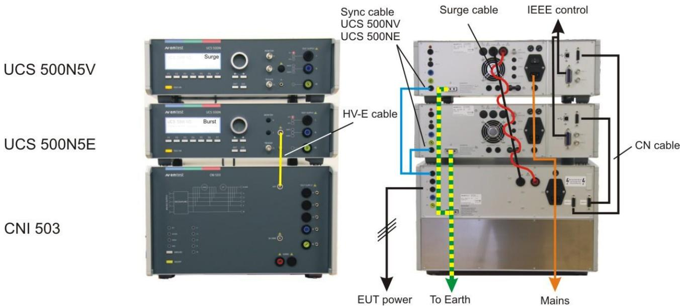
Figure 6.10: Setup and cabling
