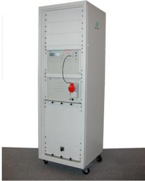
All units, the surge generator, the EFT and the coupling matrix can be installed one above the other. **The coupling matrix should than be used as central output for the EUT and should be mounted directly onto the ground reference plane. The EFT has to be installed directly over the coupling matrix to have the output connection EFT - CNI as short as possible.**
