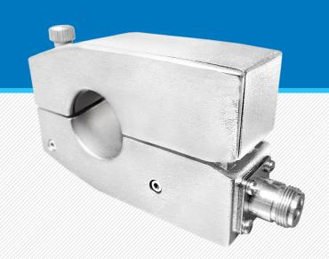
Conducted currents can be measured without making direct contact with the source conductor or metallic surface by means of clamp-on current probes.
