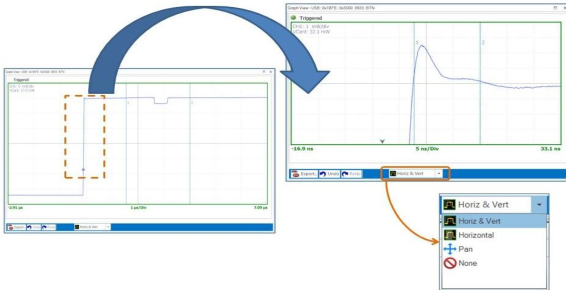
Figure 3.9 Clicking on the Trace View display and dragging will open a zoom box, releasing the mouse button will result in the trace being expanded to show the area contained in the zoom box
