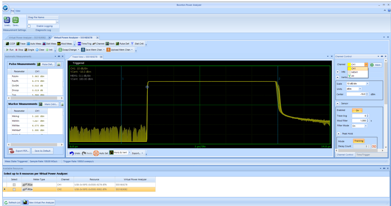
Figure 4.24 Multi-channel sensors using individual Virtual Power Analyzer (VPA) tabs. Each sensor has its own control and measurement windows associated with it which are available when the sensor VPA tab is selected.
