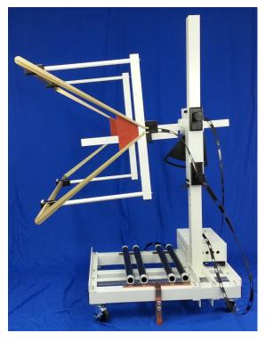
The TDK EFG-03 E-Field Generator generates controlled, high intensity fields over the operating range of 10 kHz to 100 MHz.
