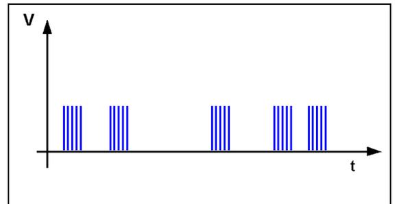
Voltage change after T by  $\Delta V$  The test voltage is increased from  $V_1$  to  $V_2$  by steps of  $\Delta V$  after the defined test time T. All limitations are the same as defined under Quick Start. The limitation of the max. generated number of spikes is related to the higher voltage of  $V_1$  or  $V_2$ .
