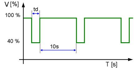
As long as the external dc supply is used, controlled by an analogue 0-10V control voltage, the test is conducted automatically. If this option is not available the manual test routine shall be used.
