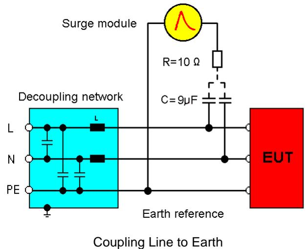
The release of the surge pulses is mostly related to a certain phase angle. The surge pulses are synchronized to the input signal at the rear Sync-connector.
