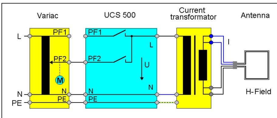
The voltage V is adjusted with a variac as long as the required antenna current is available and the related H field is generated in the center of the magnetic field antenna.
