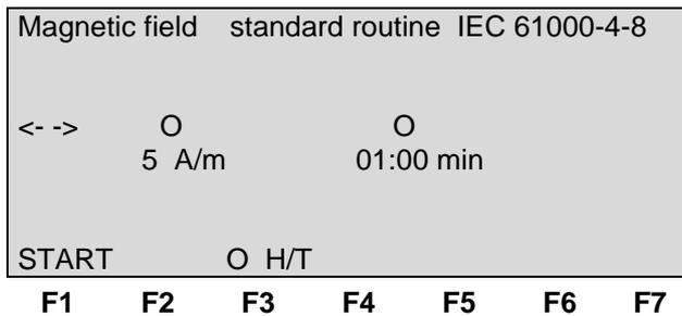
With the inc knob the values for the magnetic field strength and test duration can be changed. The actual parameter is indicated by a blinking circle.
