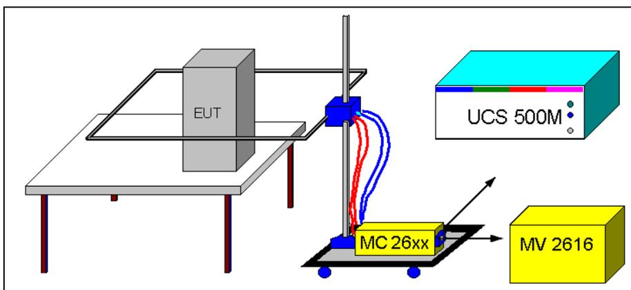
The variac, type MV 2616 may be controlled automatically via the test generator. Any equivalent variac available in the lab can be used to control the current manually. Please take care that the variac has a sufficient current capability.
