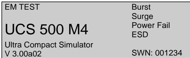
The serial number and the version number SWN are used for traceability reasons. These numbers are listed in the test reports and calibration certificates. These numbers also are listed within the test reports generated by the ISM ISO software.
