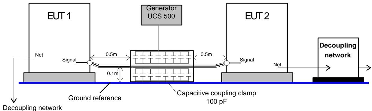
**Coupling to signal lines or lines where no galvanic contact is possible (e.g. shielded lines)**
