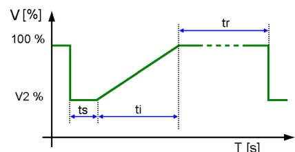
Attention: This is a new Voltage Variation function which is required in the new FDIS IEC 61000-4-11. The Voltage Variation function which is conform with the actual published IEC 61000-4-11 is available in the USER TEST ROUTINES.
