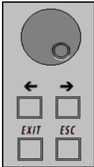
The selected parameter is blinking and can be changed by turning the knob (incr./decr.). The digit to be changed can be selected with the cursor (←→).
