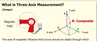
The area of magnetic influence that occurs around an object through which a current is passing is termed a magnetic field. Because the values obtained when measuring a magnetic field vary with direction due to the field's directionality, it is necessary to measure all three axes of the magnetic field.
