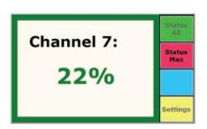
Individual Channel readings can be displayed (left) as well as all channels (below). The system will automatically adjust the size and color of the font to indicate normal or alarm situations. The pictures here just indicate a fraction of the information available on the front panel or through the Ethernet interface.
