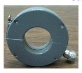
The F-65 is for laboratory and field testing. It is cabable of measuring pulse transients with risetimes of 200 picoseconds and a pulse width of 35 nanoseconds. This probe has a small outer diameter, approx. 71mm with an internal diameter of 32mm. Its transfer impedance is  $1\Omega$ from 1 MHz to 1 GHz. It can an operate up to 350 amperes of DC – 400Hz, 3 amperes of CW and 100 amperes of peak pulse.
