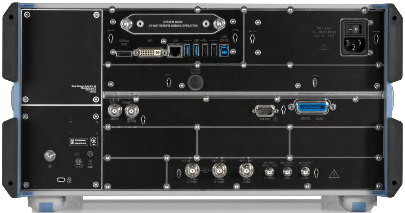
Rear view of R&S®ESW with removable hard disk drive.
