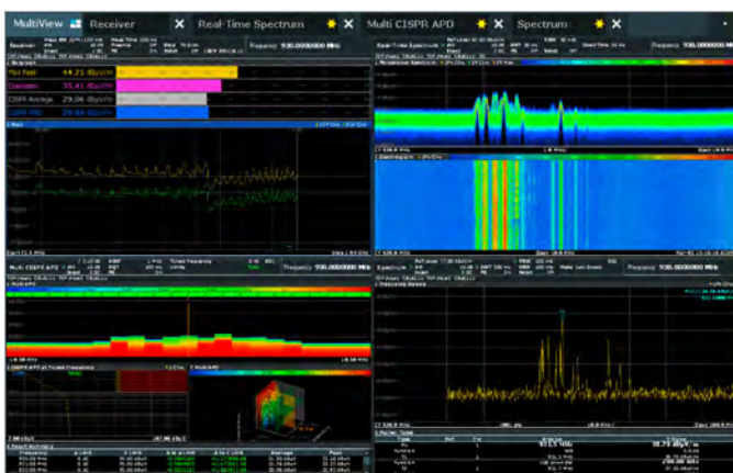
MultiView display with four operation modes shown simultaneously.
