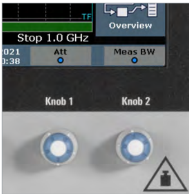
Two rotary knobs with user-assignable functions.
