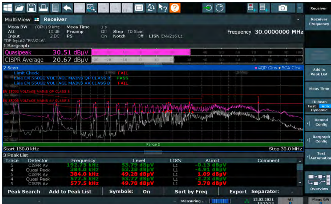
Fully automated testing of conducted disturbances with CISPR detectors without prescan.
