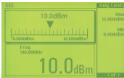
In this setup, the top half of the split display shows the analog peaking meter while the bottom display shows the same measurement with a larger character size.
