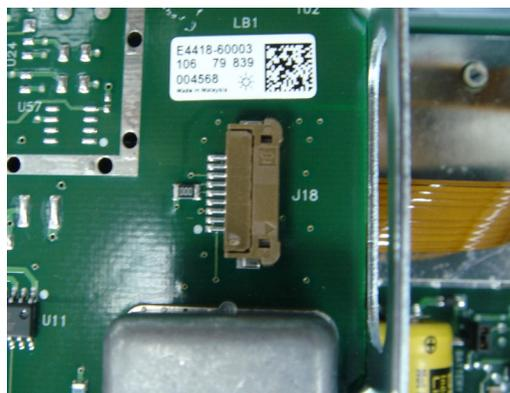
**Figure 1-5** Flex circuit connector
