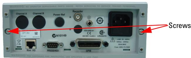
**Figure 1-1** Remove the attached screws
