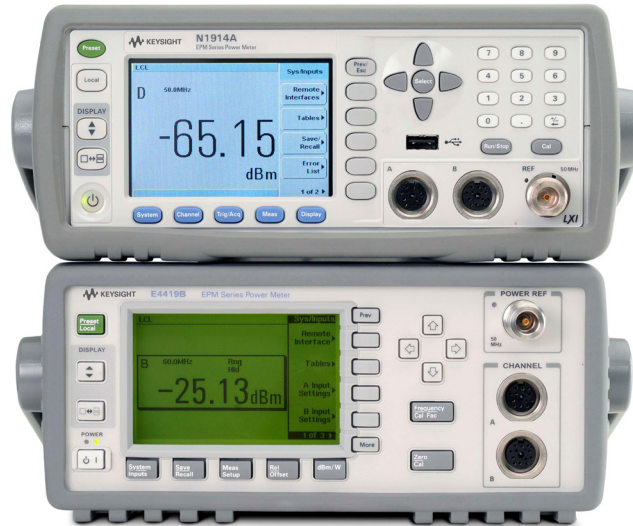
Figure 15. The N1913/1914A LCD display (top) versus E4418/4419B monochrome display (bottom)
