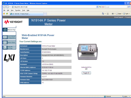
Figure 11. Instrument web browser shows instrument settings at a glance and enables remote access/control
