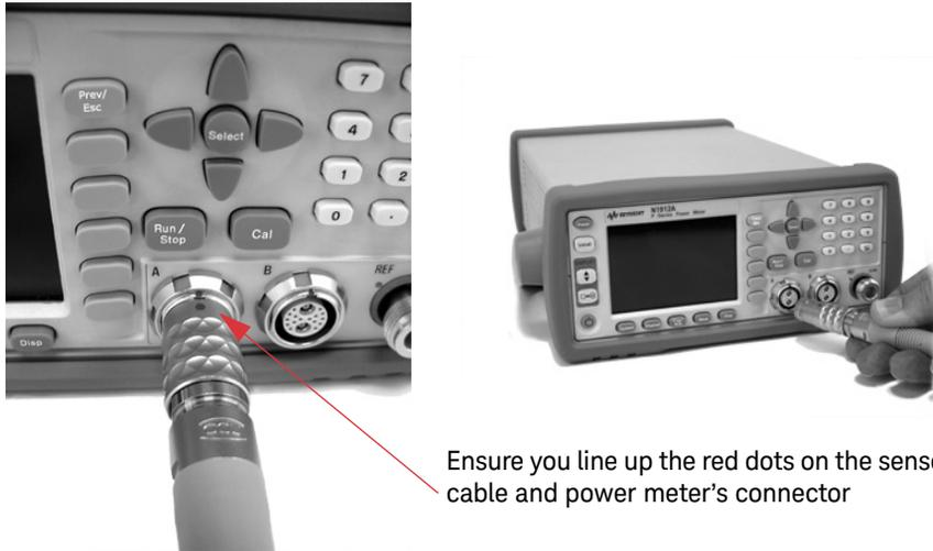
Ensure you line up the red dots on the sensor cable and power meter's connector
