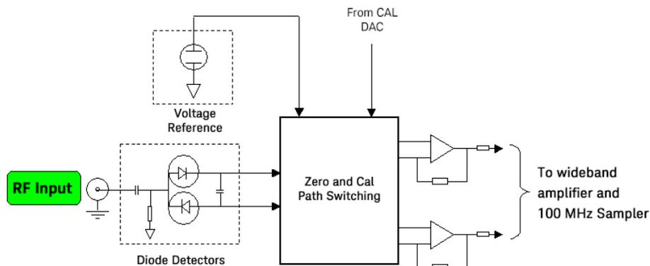
To ensure the accuracy of power measurements and improve measurement speed, the N1921/2A uses a four-dimensional (4-D) modeling technique that measures input power, frequency, temperature, and output voltage across the N1921/2A specified measurement ranges. Data from this 4-D model is generated during Keysight's initial factory calibration of the N1921/2A and stored in EEPROM.
