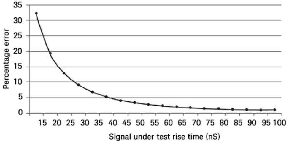
Although the rise time specification is  $\leq 13$  ns, this does not mean that the combination of P-Series power meter and power sensor can accurately measure a signal with a known rise time of 13 ns. The measured rise time is the root sum of the squares (RSS) of the signal-under-test rise time and the system rise time (13 ns):
