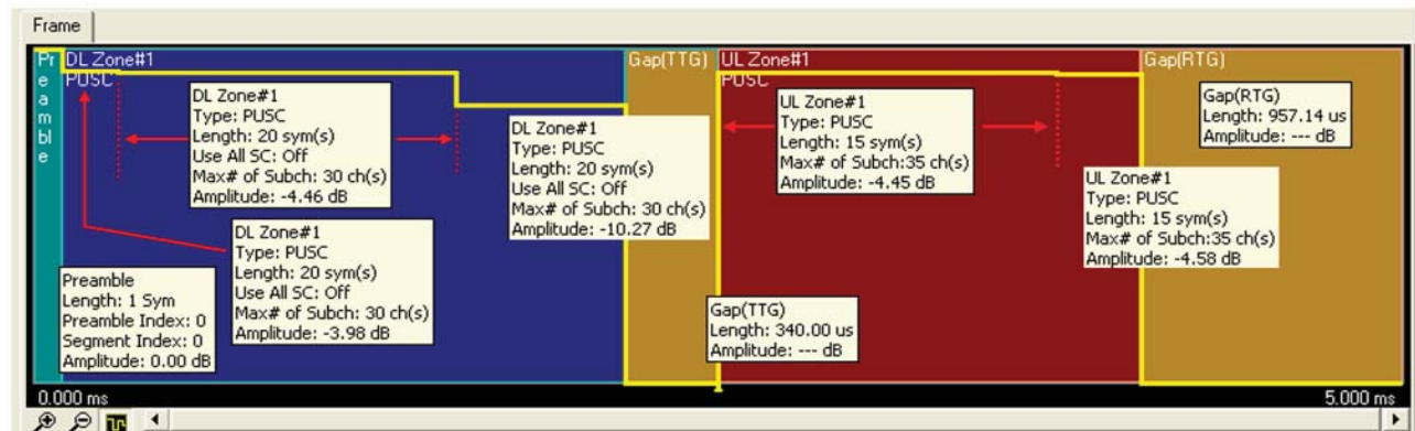
Figure 23. Frame duration (5 ms) of DL and UL waveforms captured with Signal Studio
