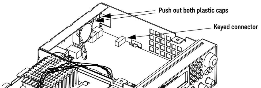
**10** Install the External Timebase Reference assembly.
