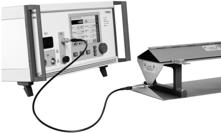
Figure 2: CDN 3425 connected to the EFT output of a NSG 3040 generator
