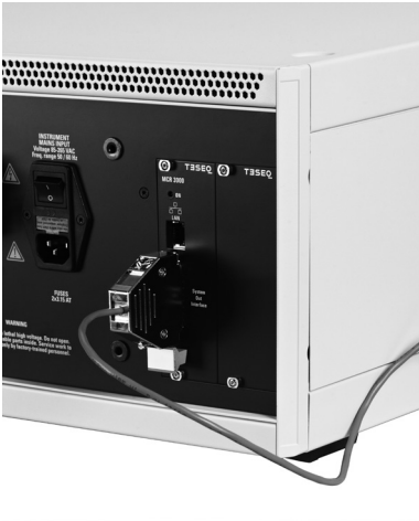
Figure 7: Connect the interlock cable to system OUT interface port of NSG 3060 series generator
