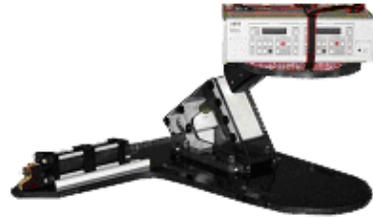
Position the manipulator in the GTEM! as far back as possible, making sure to clear the absorbers and any floor penetration panels. The mounting platforms for the different models can support the following loads:
