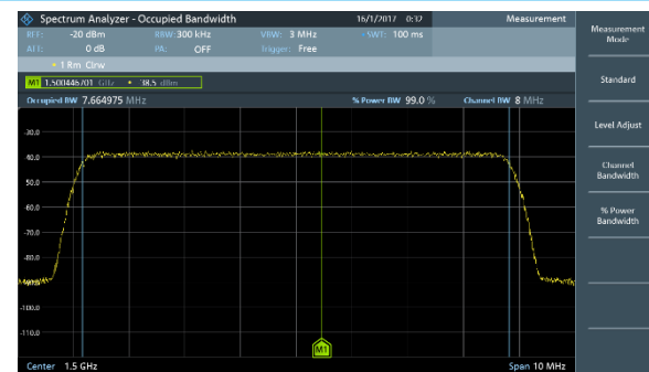
The R&S®FPC-K55 adds channel power, occupied bandwidth, spectrogram display, adjacent channel leakage ratio, spectral emission mask, spurious emissions and third order intercept.
