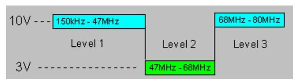
Fig 5.7: Test procedure according to IEC 61000-6-2
