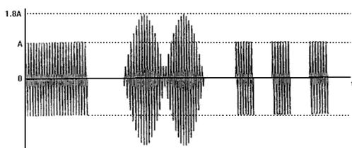
Fig 5.3 : Unmodulated 80% AM Pulse modulation
