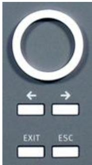
The selected parameter is blinking and can be changed by turning the knob (incr./ decrease.).
