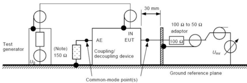
The CDN and the 150Ω to 50Ω adapter must well connect to the ground reference plane (i.e. by using copper tape).
