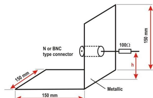
Fig 7.5 : example of reference plane dimension
