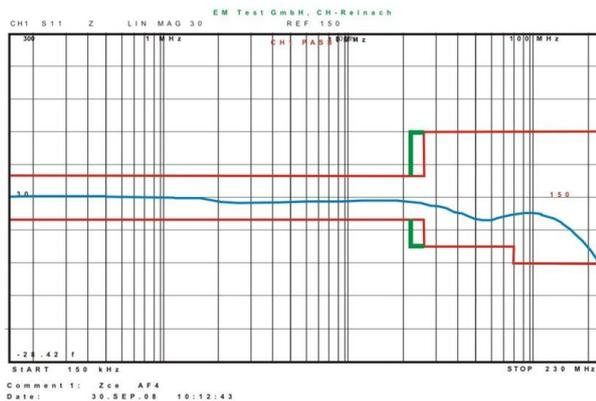
Fig 8.7 : Typical Impedance Zce of a CDN
