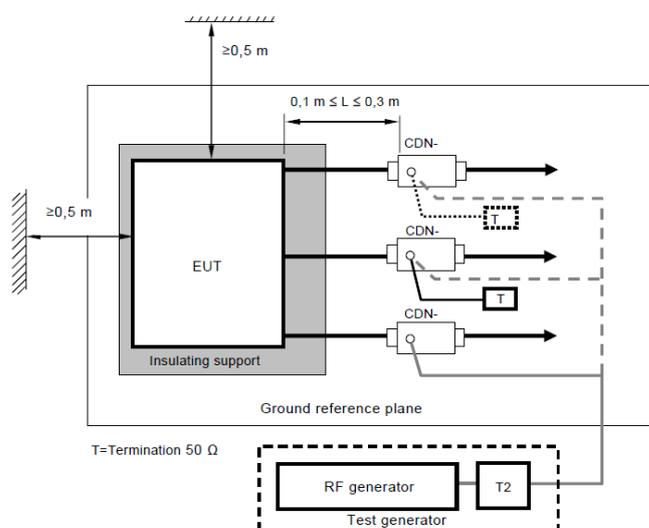
The EUT clearance from any metallic objects other than test equipment shall be at least 0,5 m.
