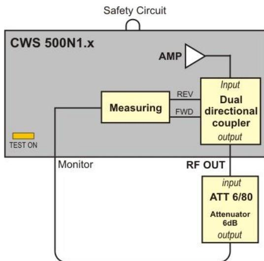
Fig 6.3 :Setup step 2 with connected 6 dB attenuator
