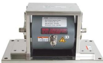
**Bulk Current Injection Clamp BCI type F-120-9A**
