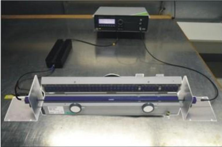
Fig 7.4 : Calibration setup with EM Clamp
