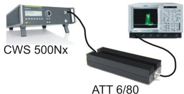
Fig 6.1 Setup for a function test
