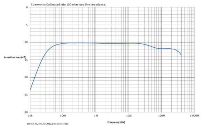
Fig 8.8. : Typical insertion loss of a CDN
