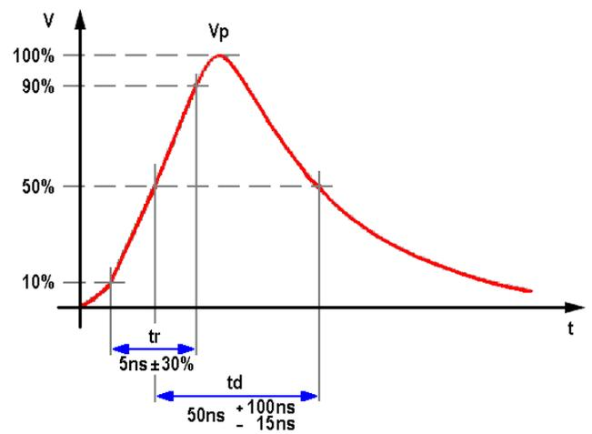
Waveform definition into 1000Ω
