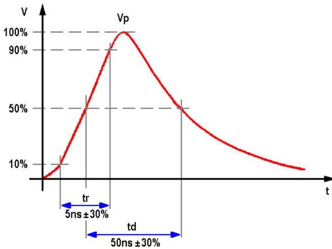
Waveform definition into 50Ω
