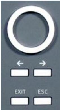
The selected parameter is blinking and can be changed by turning the knob (incr. /dec.). The takeover of the input value occurs after about 500ms encoder downtime. This allows the operator a brief check of the correct input value.
