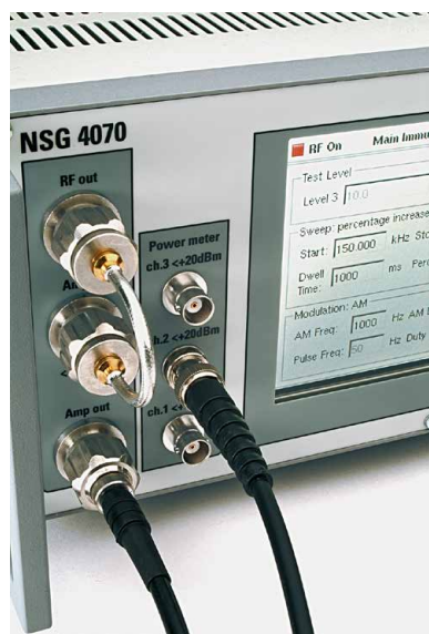
NSG 4070 front panel with RF ports
