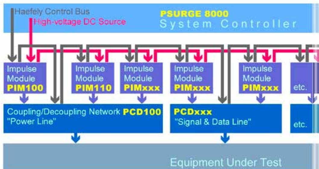
The surge platform hardware comprises a control unit with access to maximum 99 modules interconnected on the HAEFELY bus.
