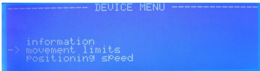
2. Navigate to “information” and press “ENTER”. The device type, the serial number and the firmware version is shown.
