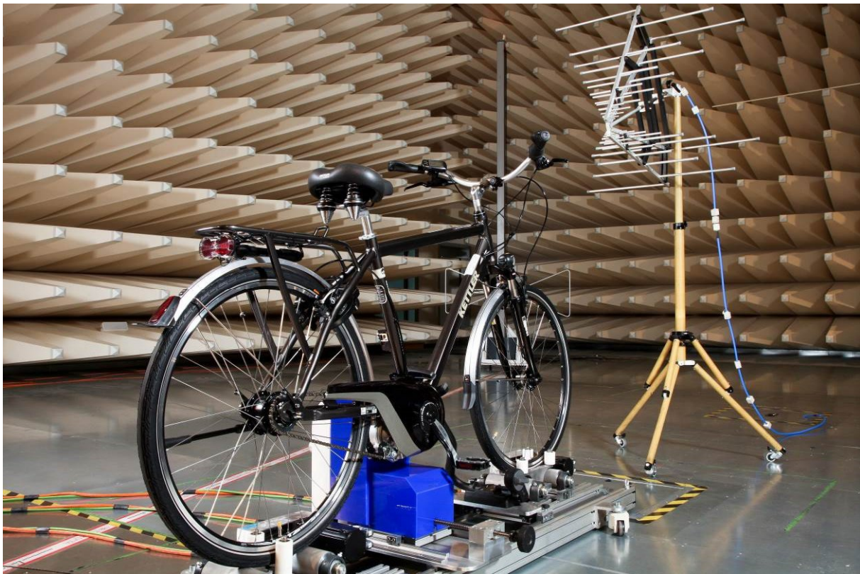
Fig.: E-Bike Dynamometer in the field at VDE
