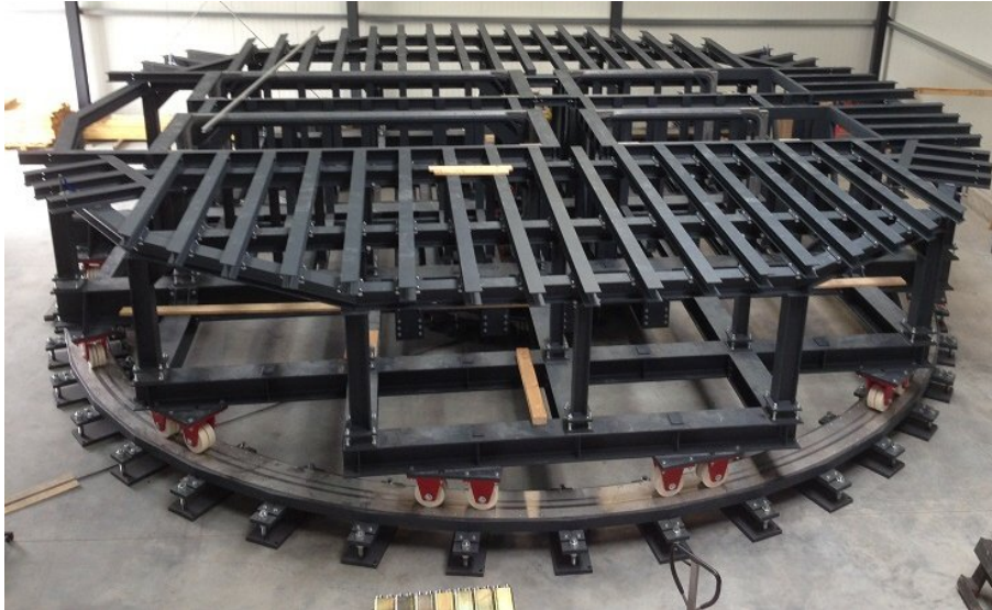
Fig.: Turntable structure made of solid welded steel
