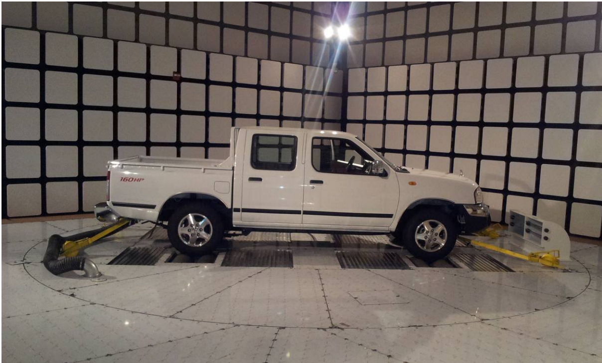
Fig.: Turntable with integrated dynamometer at Nissan, USA
