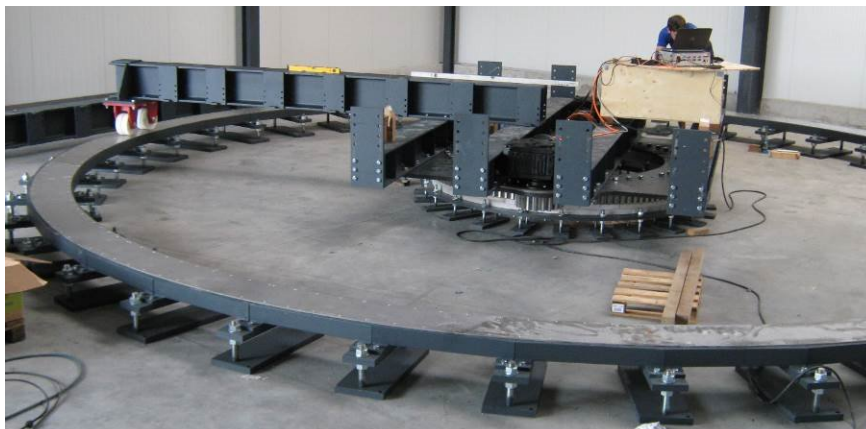
Fig.: Height adjustable runway
