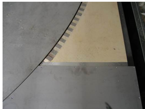
Fig.: Contact system between the turntables and to the ground plane
