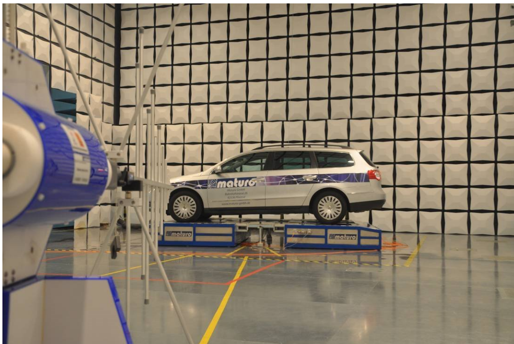
Fig.1: Test setup for measurements from 30 MHz to 1 GHz
