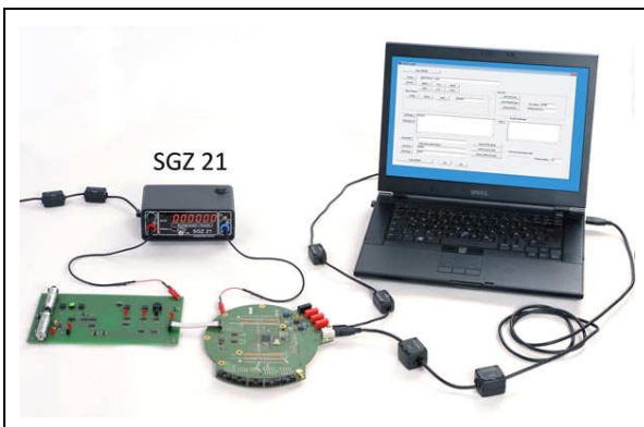
Figure 27: Injection of disturbance current via a two-pole connection and the connector of two modules. Contact is made to ground of each of the modules.
