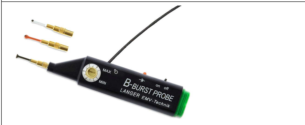
Figure 49: Magnetic field probe with exchangeable heads and an optical fibre from the S2 set.
