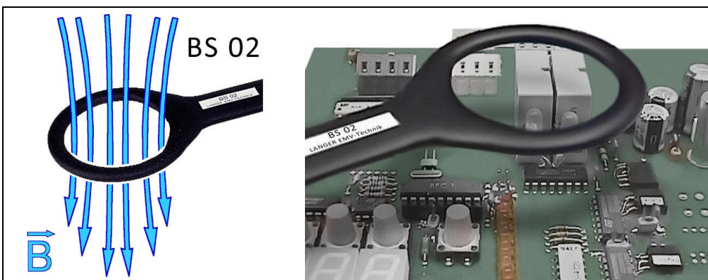
Figure 36: BS 02 field source with a large field beam to apply a magnetic field to conductor loops of around 10 cm.
