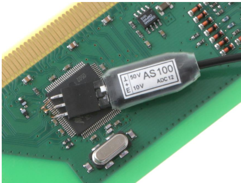
Figure 9 AS 100 connected to the EUT; position the AS 100 on the IC package if there isn't enough free space above GND
