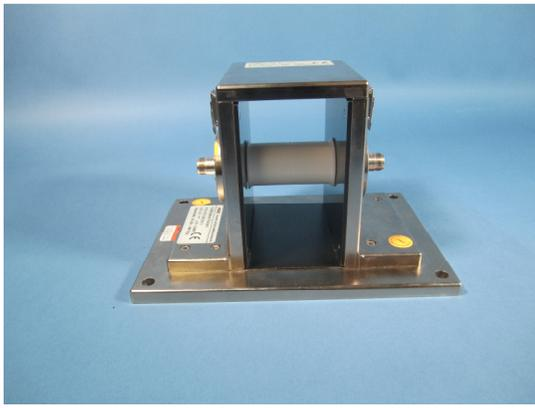
Injection Probe Calibration Fixtures are a part of the test equipment required by most of the Bulk Current Injection test procedure specifications. The FCC-BCICF-1 calibration fixture allows the user the quickly and easily calibrate the injection probe prior to performing compliance testing.
