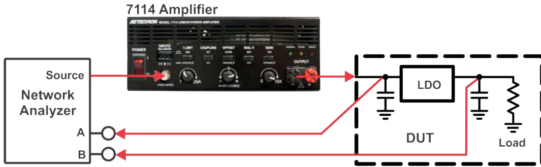
Figure 6.16 – LDO PSRR Measurement, Testing Setup
