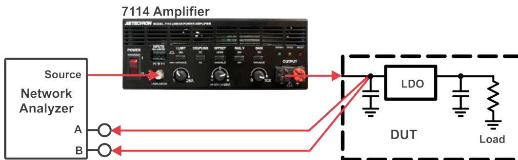
Figure 6.15 – LDO PSRR Measurement, Calibration Setup
