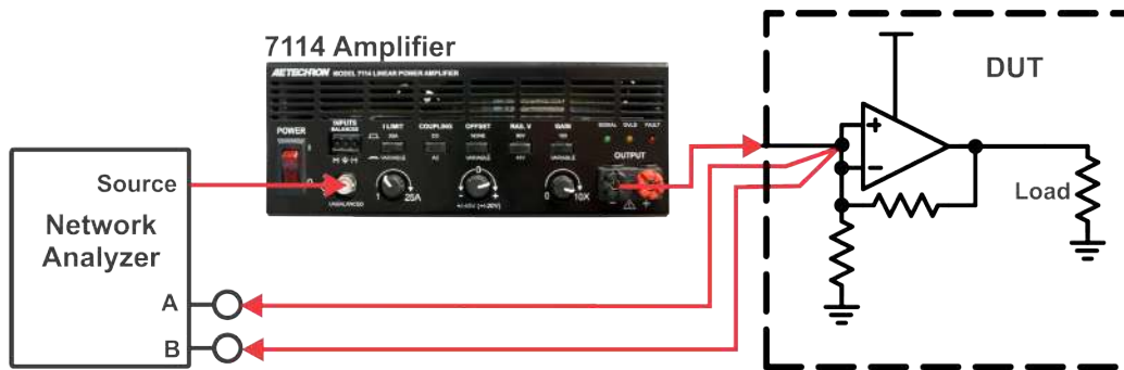
Figure 6.20 – Amplifier CMRR Measurement, Calibration Setup
