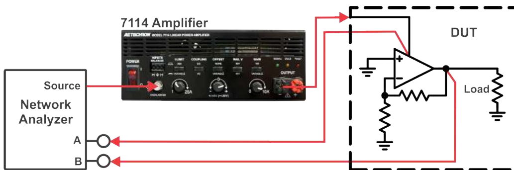
Figure 6.19 – Amplifier PSRR Measurement, Testing Setup
