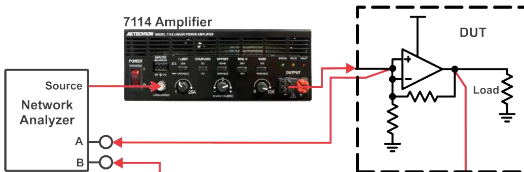
Figure 6.20 – Amplifier CMRR Measurement, Testing Setup
