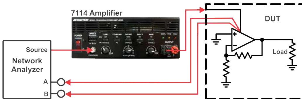
Figure 6.18 – Amplifier PSRR Measurement, Calibration Setup
