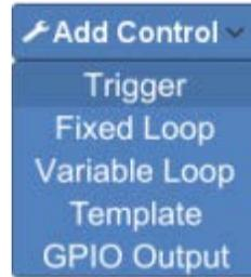
When you choose a control from the Add Control drop-down menu, an icon representing that control type is added to the active window, and a form containing the available settings for that control opens below the active test display. See the individual entries in this Help system for more information about the settings available for each control type.
