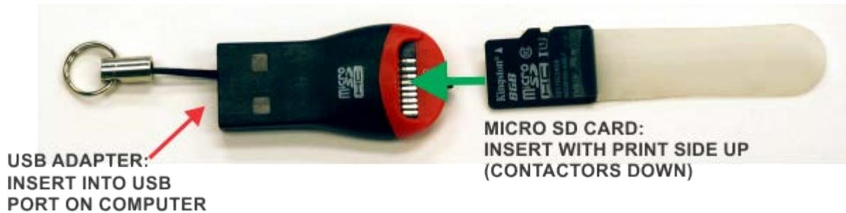
The microSD card contains the SWG Setup.exe file that is used to install the remote access SWG program on a Windows computer. For more information, see the topic "*DSR 100-15 via Network.*"
