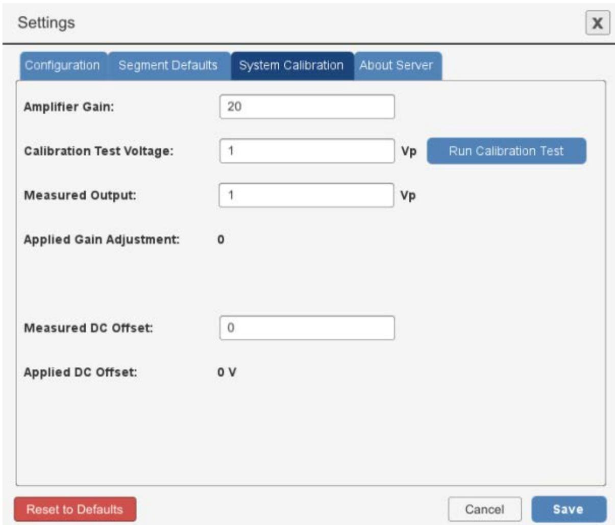
The screenshot shows a 'Settings' window with a close button (X) in the top right corner. Below the title bar are four tabs: 'Configuration', 'Segment Defaults', 'System Calibration' (which is selected and highlighted in blue), and 'About Server'. The 'System Calibration' tab contains several input fields and buttons:
