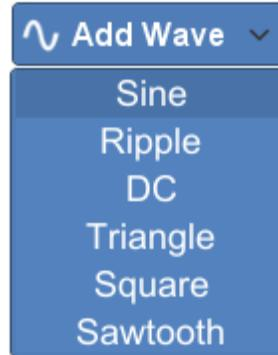
When you choose a waveform from the Add Wave drop-down menu, the default waveform of that type is added to the active window. Click on the tab or the waveform in the display to open the Properties form containing the available property settings for that waveform. See the individual entries in this Help system for more information about the settings available for each waveform type.
