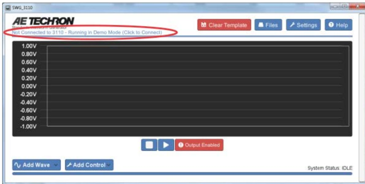
You can use the Add Wave and Add Control buttons to create a waveform sequence. In addition, you can load existing tests from the Standard's Library to use as a template or to edit and save as a new test file.
