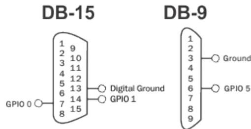
Each GPIO port can be configured as an Input or an Output.
