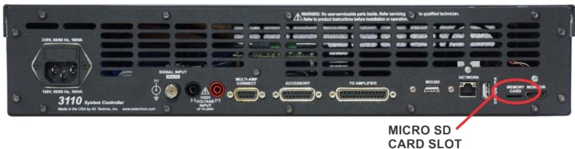
3. Remove the micro SD card from the USB adapter and insert the card into the Memory Card slot. Be careful when installing the card to insert the card with the printed side UP. The card must also be inserted in a straight line directly into the card slot. If the card is inserted at an angle, it may miss the internal card slot and be inaccessible from your DSR 100-15 unit.
